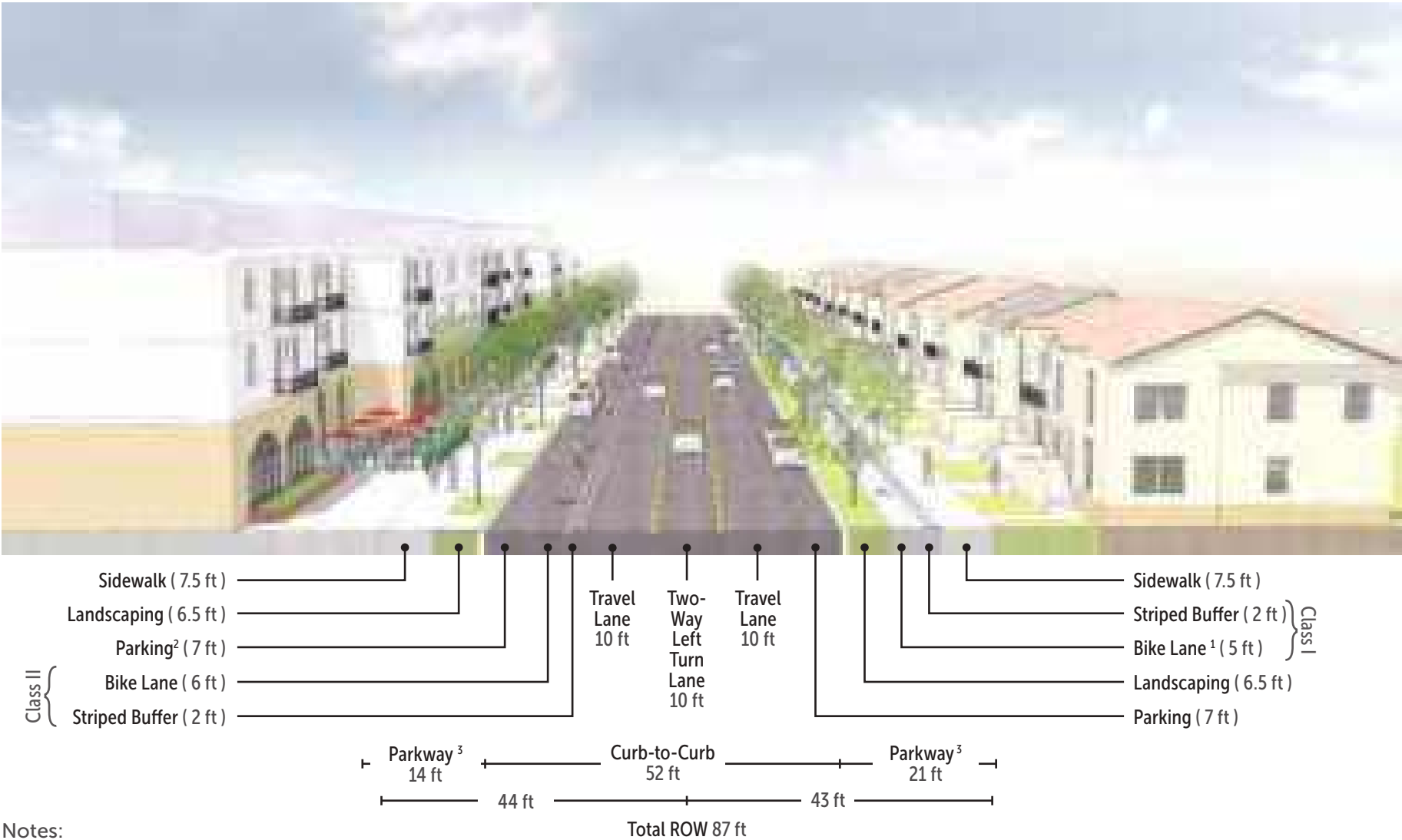
Figure 4.11 – Modified Cross-Section for 2-Lane Collector with Two-Way Center Left Turn Lane, Class II Bike Lane with Buffer on West Side, and Class I Bike Lane with Buffer on East Side
