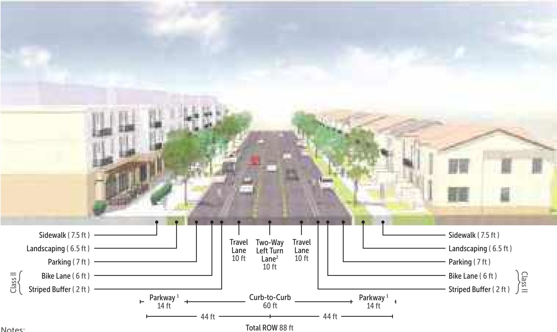
Figure 4.9 – Modified Cross-Section for 2-Lane Collector with Two-Way Center Left Turn Lane with Class II Bike Lanes with Buffer
