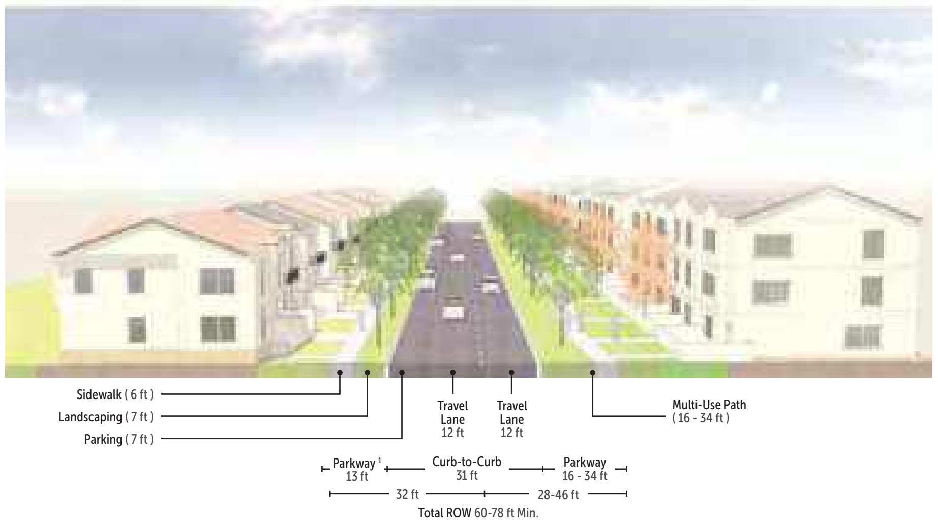
Figure 4.17 – Modified Cross-Section for 2-Lane Collector Street with Multi-Use on One Side (Exterior Side)
