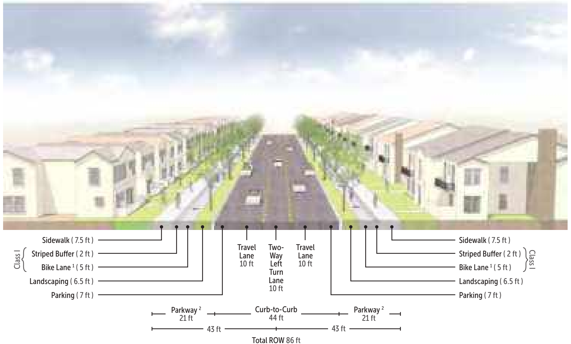
Figure 4.10 – Modified Cross-Section for 2-Lane Collector with Two-Way Left Turn Lane and Class I Bike Path
