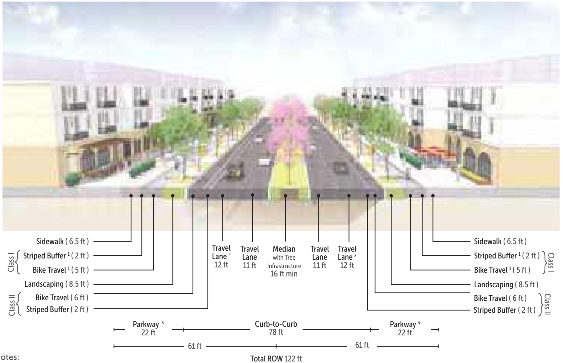
Figure 4.6 – Modified Cross-Section for 4-Lane Urban Collector with Class I Bike Paths and Class II Bike Lanes
